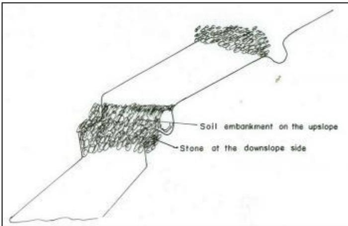
**Figure 55: Example of bench (bund/banquette) terraces (source: [www.wocat.net](http://www.wocat.net)).**
