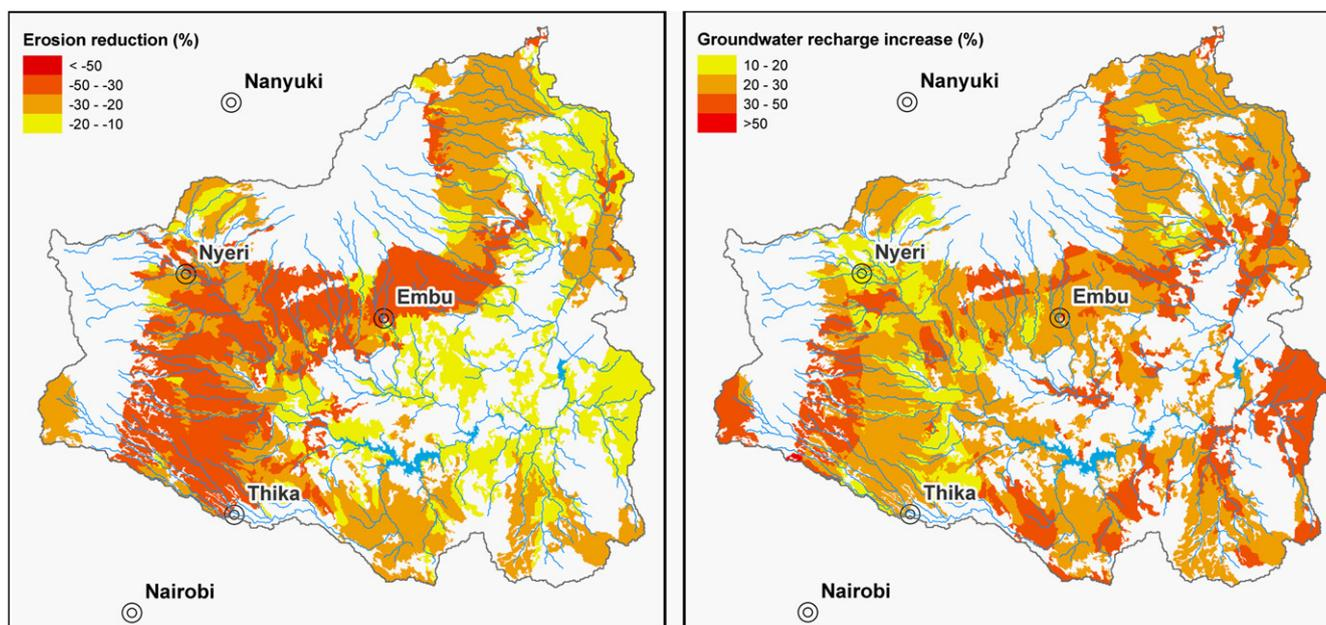
Fig. 5. Spatial distribution of relative erosion reduction (left) and the increase in groundwater recharge (right) for the vegetative contour strips scenario, based on yearly averages.
