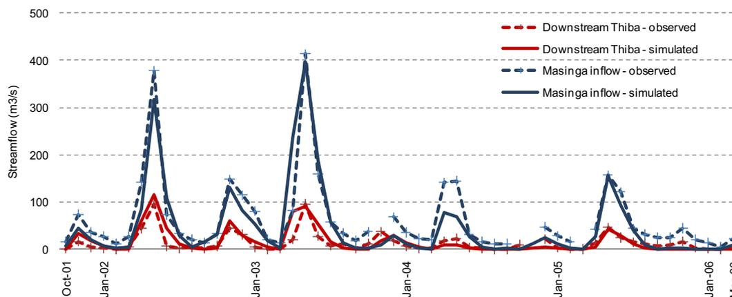
Fig. 3. Simulated and observed inflow at downstream points of two major catchments of the basin.
