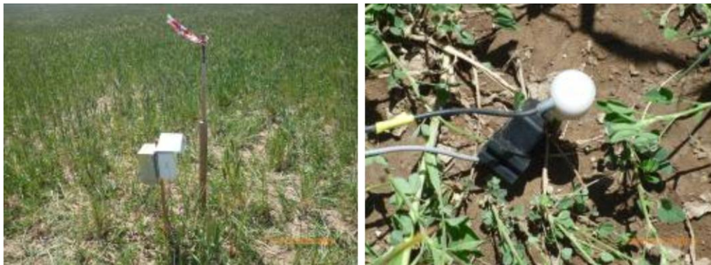
Figure 5. Elementary Sample Unit with dataloggers (left) connected to PARAMETER-PASTIS coupled system (right).
