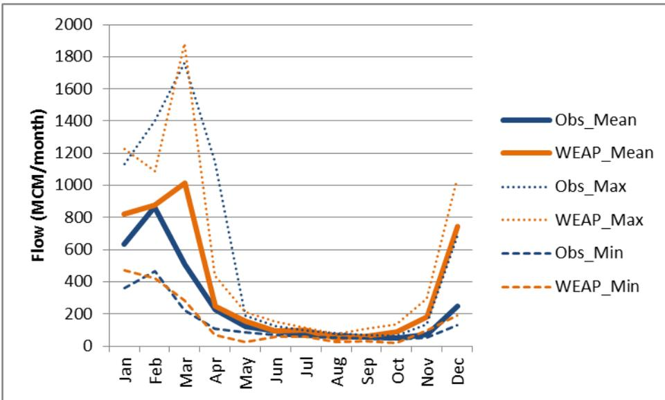
Figure 10. Validation of the WEAP model: outflow observed and modeled to Indian Ocean.
