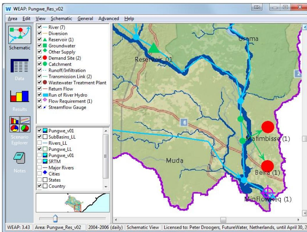
**Figure 24. The WEAP model used as an O-DSS (Operational Decision Support System) to explore operational rules for a proposed reservoir.**
