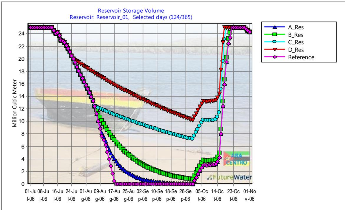
**Figure 25. Different operations of the reservoir and its impact on reservoir volume as explored using WEAP as an O-DSS (Operational Decision Support System). Data used for two historic years 2005 (top) and 2006 (bottom) as demonstration.**
