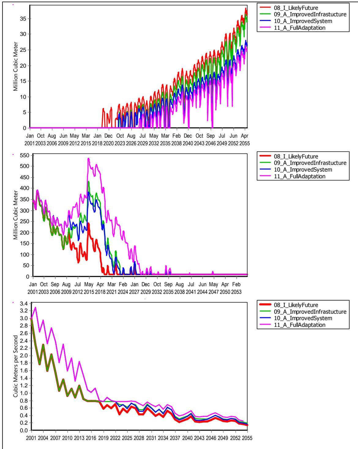
**Figure 21. Effectiveness of adaptation scenarios on unmet demand (top), reservoir volumes of P. Libombos (middle) and streamflow at outlet point of Umbeluzi (bottom).**
