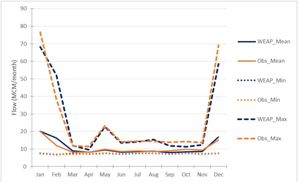
Figure 15. Observed and simulated outflow of the Pequenos Libombos reservoir.
