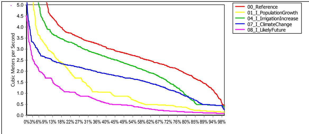
**Figure 20. Annual Umbeluzi streamflow at outlet point into Indian Ocean (top) and exceedance probability of Umbeluzi streamflow at outlet (bottom), expressed as % of months, for the Impact Scenarios.**
