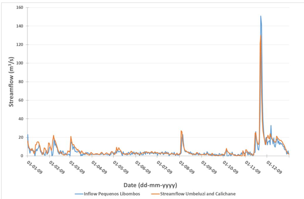
**Figure 36. Comparison of inflow into Pequenos Libombos and streamflow of Umbeluzi and Calichane for 2009.**
