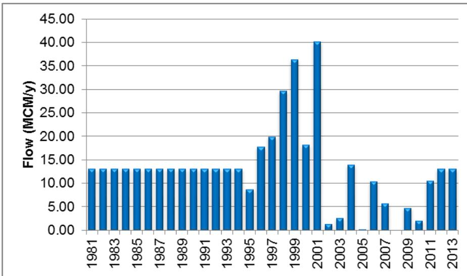
Figure 33. Total yearly streamflow for Calichane from 1981-2013 measured at gauging station E-0019H.
