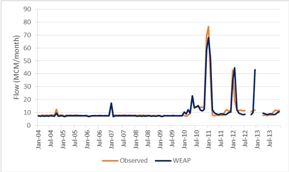
Figure 16. Observed and simulated monthly outflow of the Pequenos Libombos reservoir.
