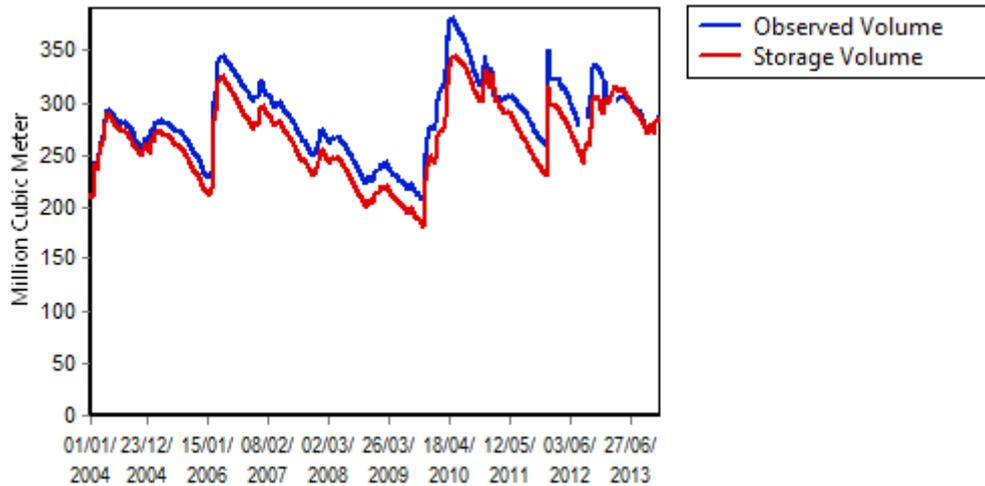
**Figure 37. Observed reservoir volume (blue line) and simulated reservoir volume of the uncalibrated model (red line) from 2004 to 2013.**
