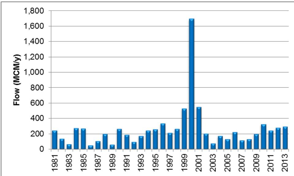
Figure 32. Total yearly streamflow for Umbeluzi from 1981-2013 measured at gauging station E-0010H.
