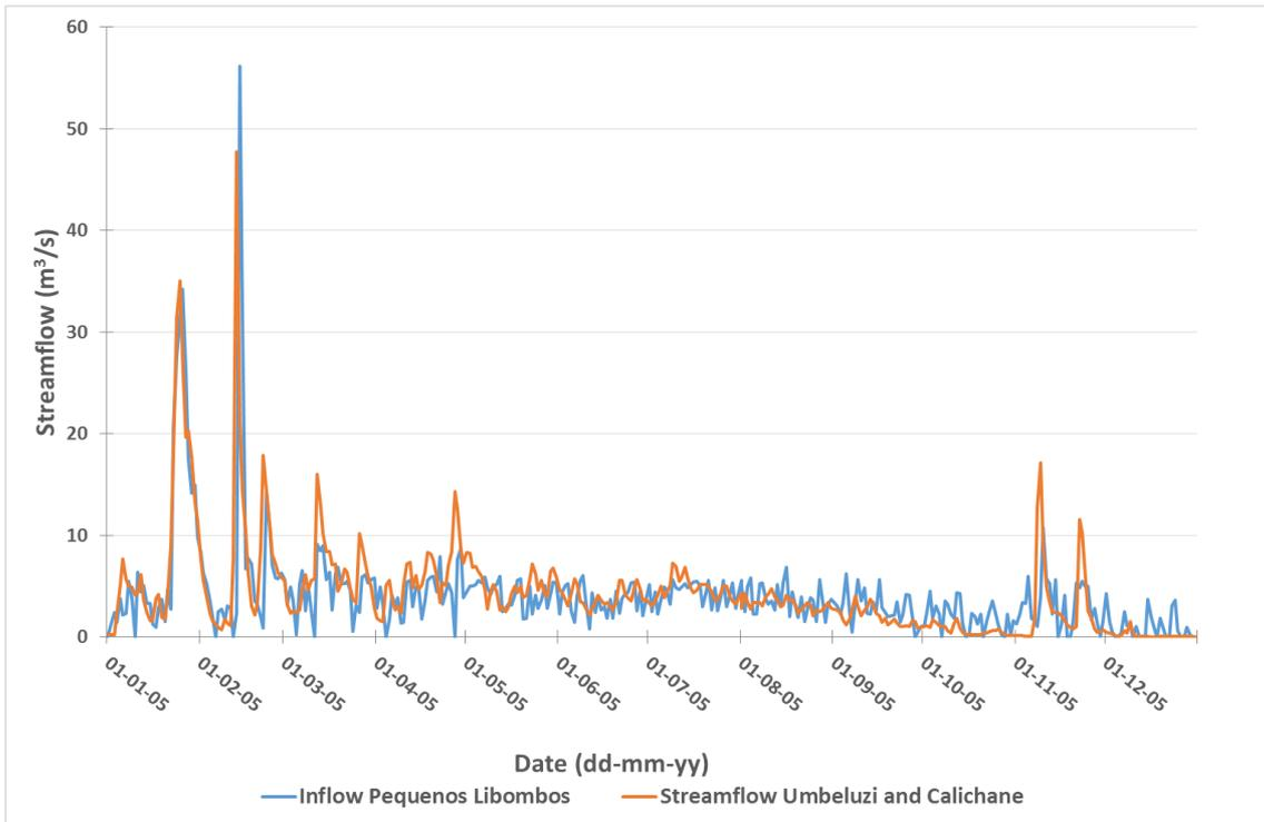
**Figure 35. Comparison of inflow into Pequenos Libombos and streamflow of Umbeluzi and Calichane for 2005.**
