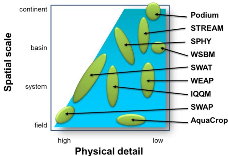
**Figure 4: Relation between spatial scale and physical detail in water allocation tools. The green ellipses show the key strength of some well-known models. (Source: Droogers and Bouma, 2014)**
