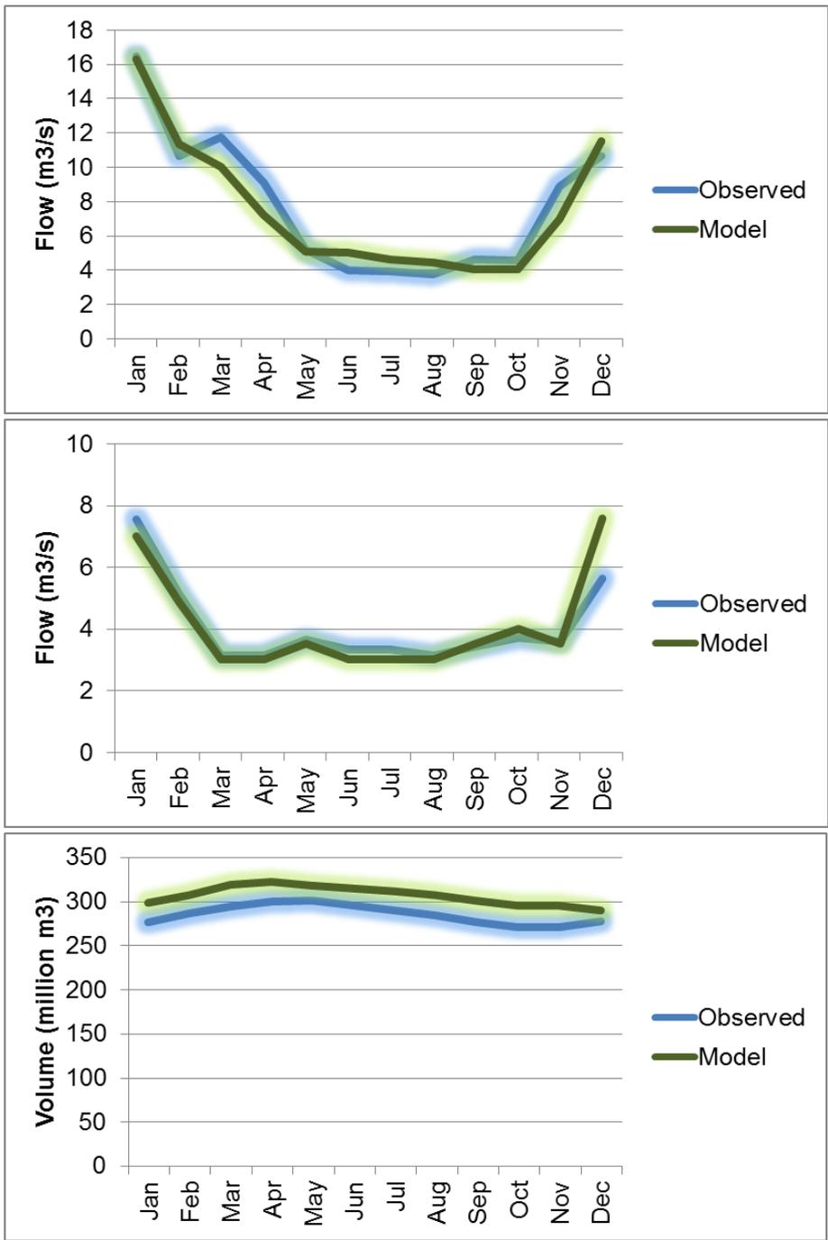
Figure 10. Observed and modelled inflow into Pequeños Libombos (top), outflow from Pequeños Libombos (middle), and volume of Pequeños Libombos (bottom).
