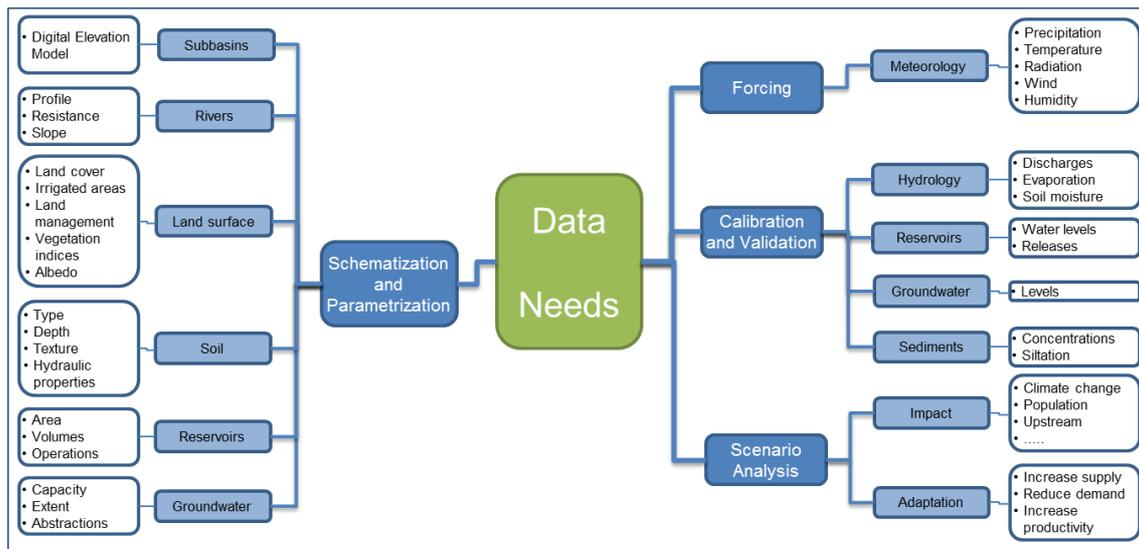
Figure 26. Overview of data needs to build water allocation models.
